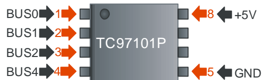
Figure 5. Wiring diagram for TC97101P EEPROM
