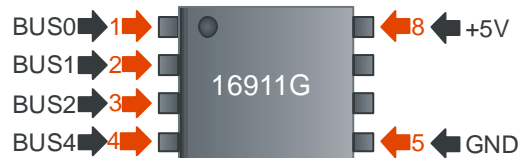
Figure 4. Wiring diagram for 16911G EEPROM
